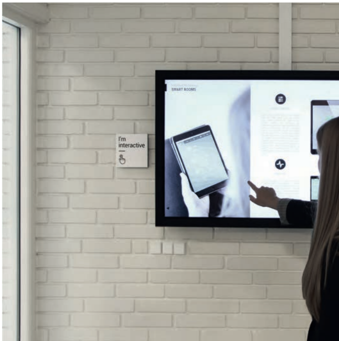
9 3XN, Green Solution House, Rønne, Denmark, 2012 The Smart Room collective monitoring of the Green Solution House by GXN with Autodesk Research is designed to allow guests to visualise the impacts of their use of the building and to see real-time building performance data relating to energy, light, air and water use.
