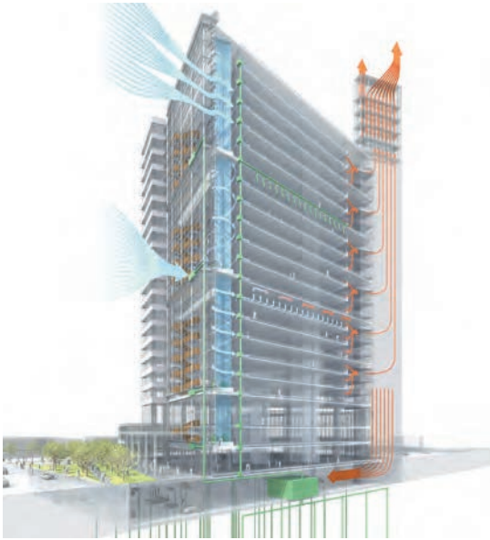
5 KPMB Architects, Smith Carter Architects and Prairie Architects, Manitoba Hydro Downtown Office, Winnipeg, Manitoba, Canada, 2009 A drawing of the seasonal climate concept.
