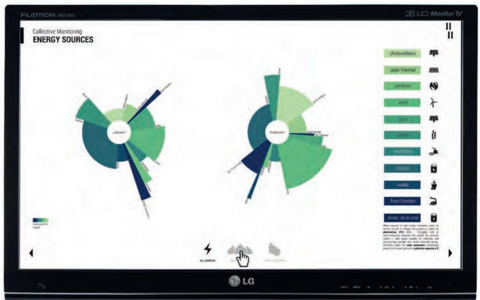
10 GXN and Autodesk Research, collective monitoring at the Green Solution House, Rønne, Denmark, ongoing research The visualisation dashboard application was designed to show guests the sources of their energy use in real time, for example what proportion of their energy use came from renewable sources.
